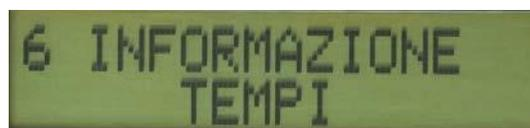
Times information is the voice of the menu that visualize the summary of the settings made by the pyrotechnician. In case of a constant, fast or slow series, the screen of times information indicate the type of series set, the time interval between the ignitions or the total duration of the series an in addition the number of ignitions of the series.
