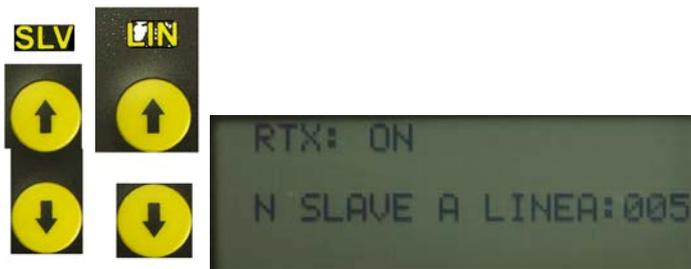
Note 1: remember that the number of Slaves per line is always equal at the number of posts present in the show and that this setting will be used from the Master at the moment of the execution of the show and in the system test phase.
