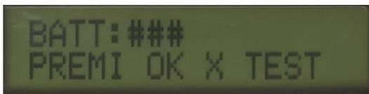
The second line "Push OK to TEST" invite the pyrotechnician to proceed to the test and to the other features of the menu.
